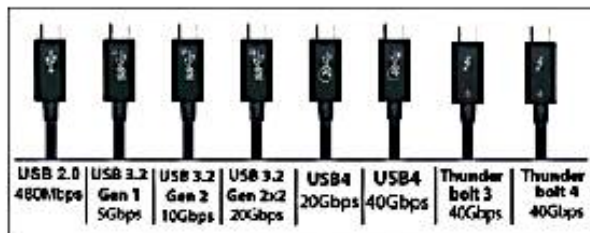
Figure 1.23: USB generations based on data transfer rate
