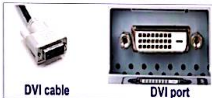
Figure 1.37: DVI cable and a DVI port
