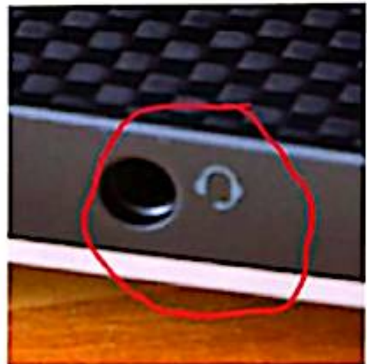
Figure 1.49: Single multi-functional audio port
