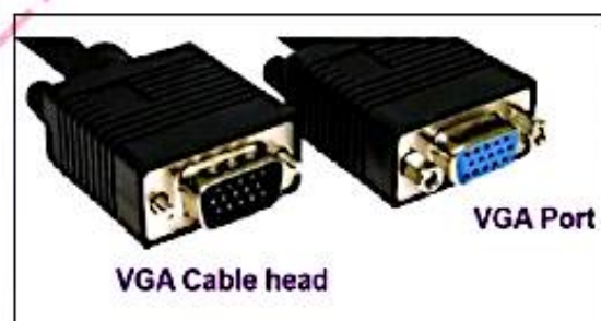
Figure 1.42: VGA port and its corresponding connector
