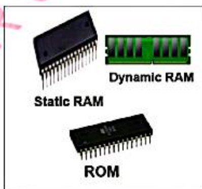
Figure 1.8: Primary storage devices (ROM and RAM)
